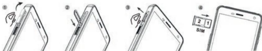
›› Insert the SIM card into the slot. The device has a slot for two SIM cards or for one SIM card in combination with a microSD card.
