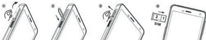
›› Insert the microSD card into the slot. The device has a slot for one SIM card in combination with a microSD card up to 128 GB, also see section “Insert/remove SIM card”.
